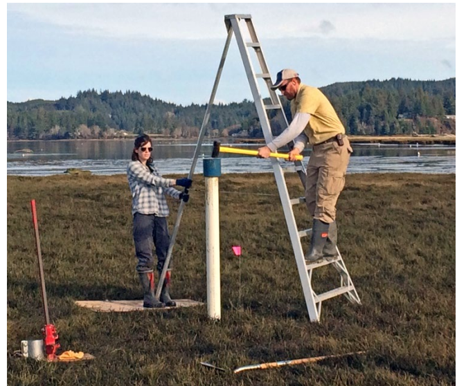
Researchers install a soil corer in the Alsea Bay high marsh to study blue carbon burial in Oregon's tidal wetlands. Photo by Oregon Sea Grant (2017a).
